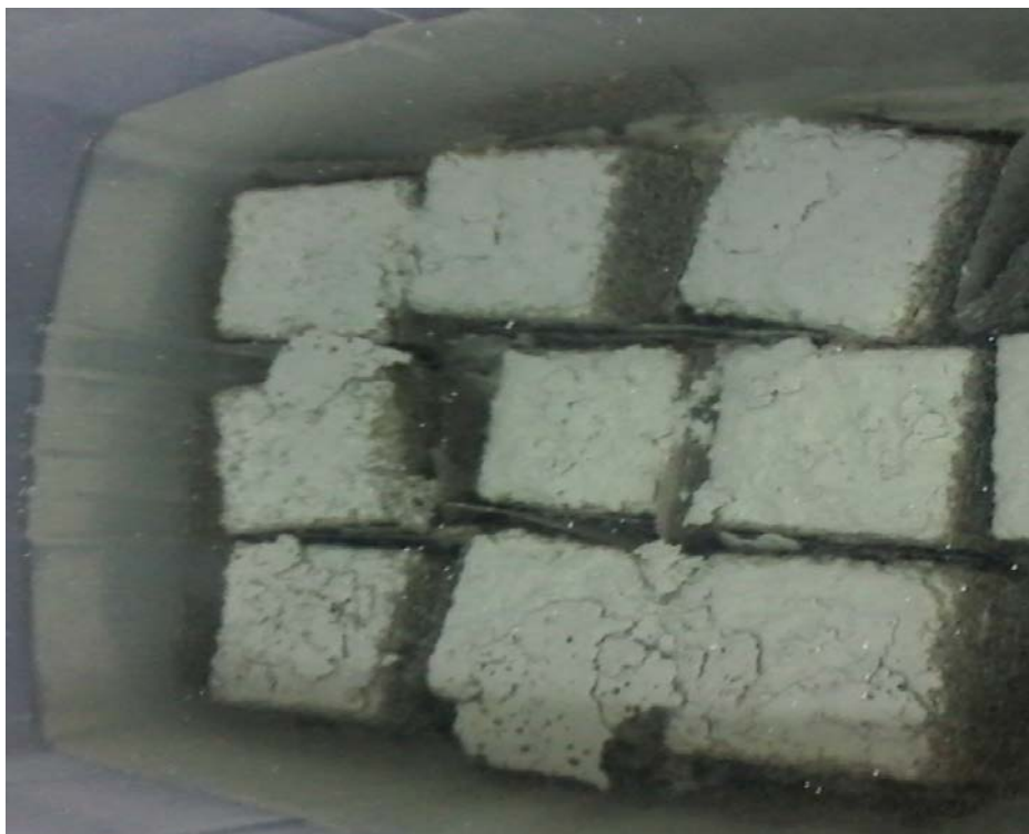
Figure (25) the surface case of blended concrete withhyb. (NS +NC) immersion in sulfate for 12 month
