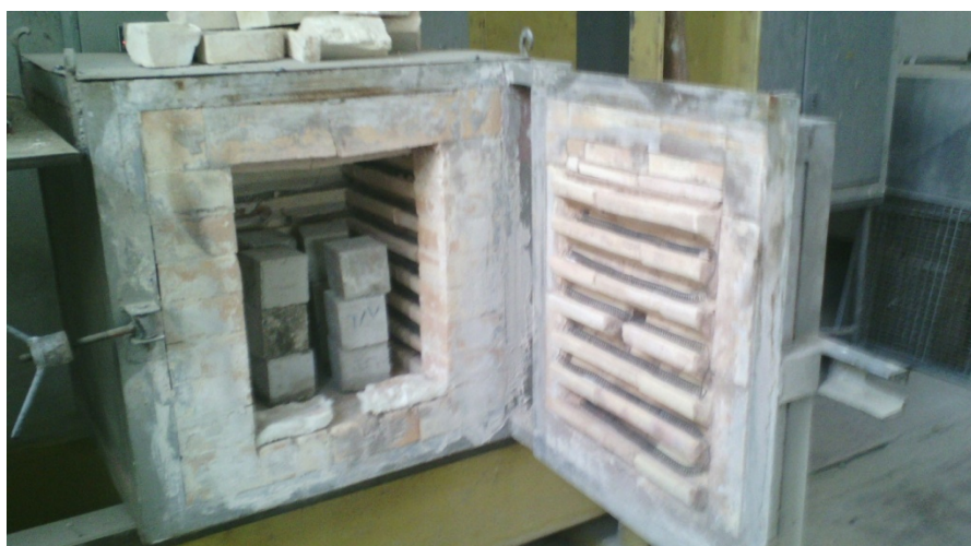
Figure (5) the concrete specimens inside the furnans to exposure to the fire
