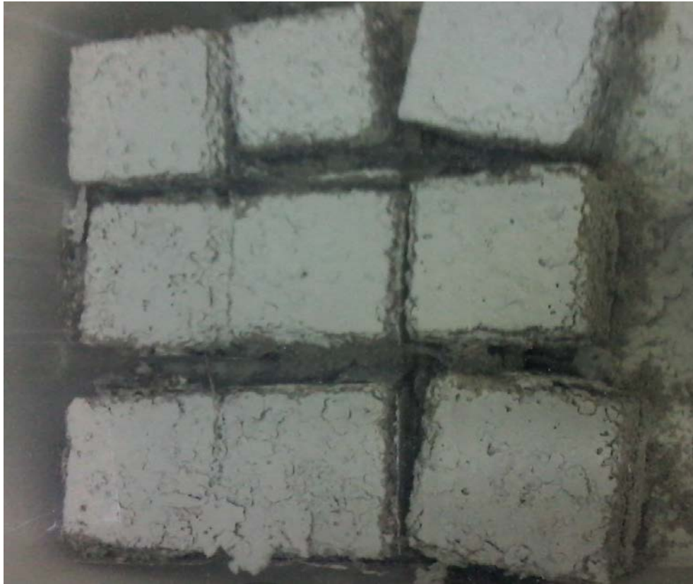
Figure (23) the surface case of blended concrete with nanoclay immersion in sulfate for 12 month
