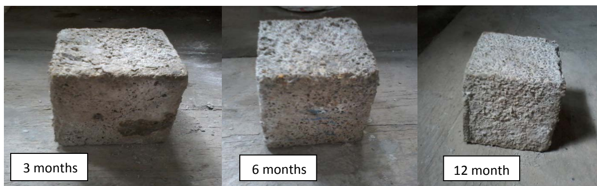
Figure (22) the surface deterioration of specimens after immersion in magnesium sulfate for 3, 6, 12 months
