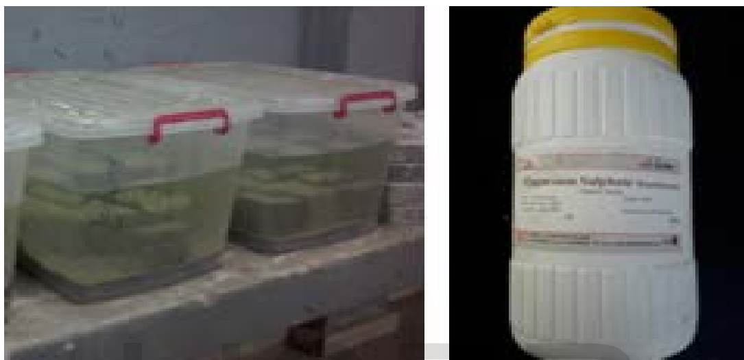
Figure (6) the specimens immersed in magnesium sulfate and the salt bottle
