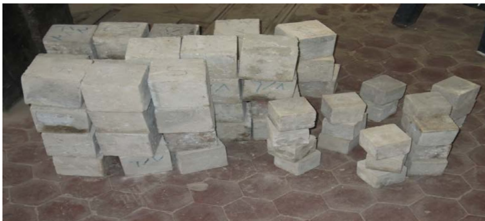
Figure (3) the concrete specimens with dimension 10x10x10 cm
